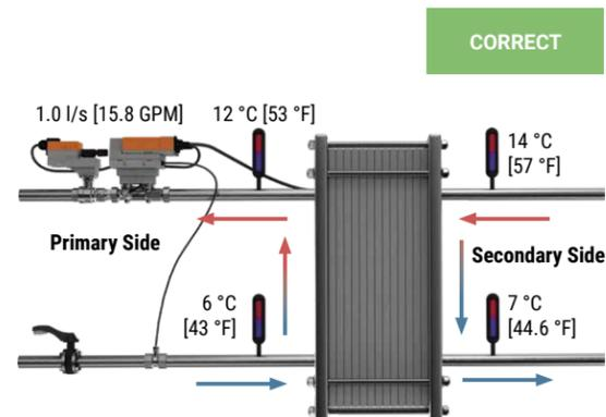
Figure 79: Dynamic balancing with Delta T Monitoring
