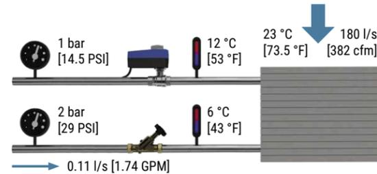
Figure 84: FCU at design operation
