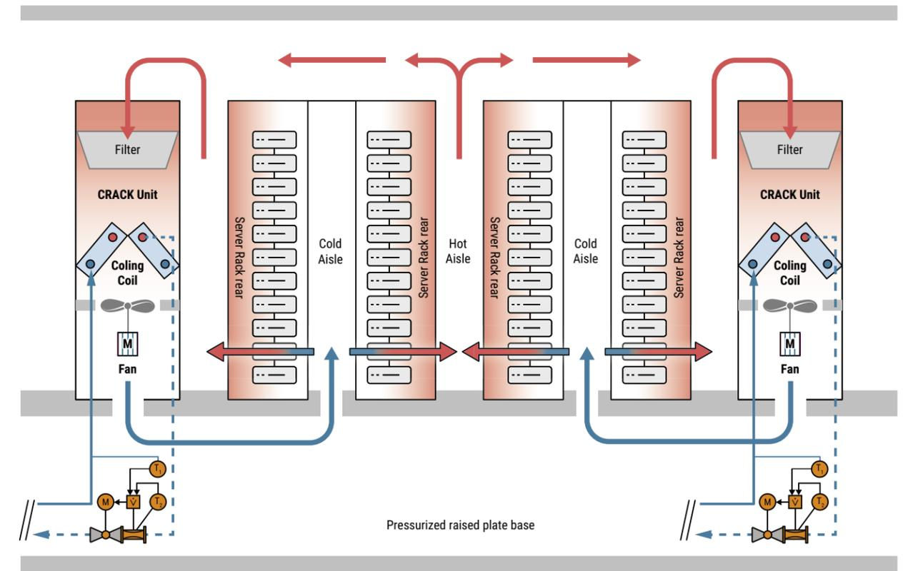
Figure 123: Schematic of a CRAC Unit including the air flow cycle to / from the racks
