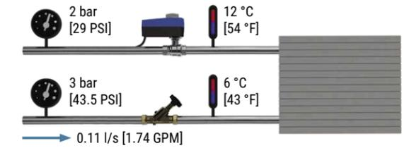
Figure 105: FCU in cooling condition
