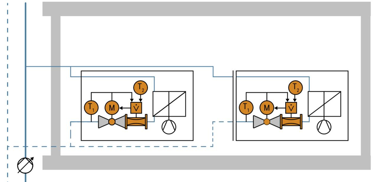
Figure 82: Typical fancoil application in a single room with one EV per fancoil
