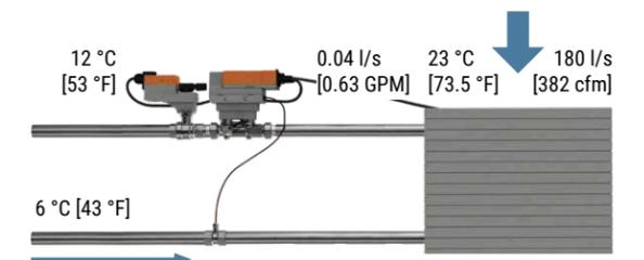
Figure 88: FCU with delta T optimized valve flow
