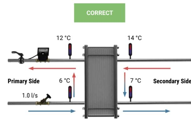
Figure 74: Typical design flow (cooling application)
