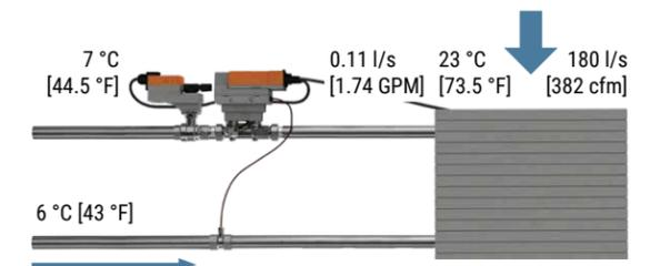
Figure 87: FCU without water overflow
