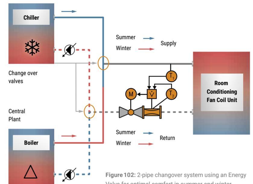
Figure 102: 2-pipe changover system using an Energy Valve for optimal comfort in summer and winter
