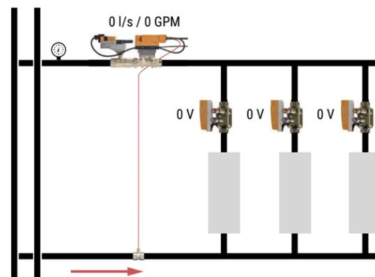
Figure 120: Dynamic Balancing with Monitoring
