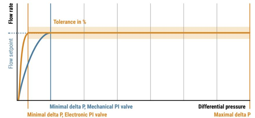
Figure 13: Electronic PI valves can maintain flow at lower delta P than mechanical PI valves
