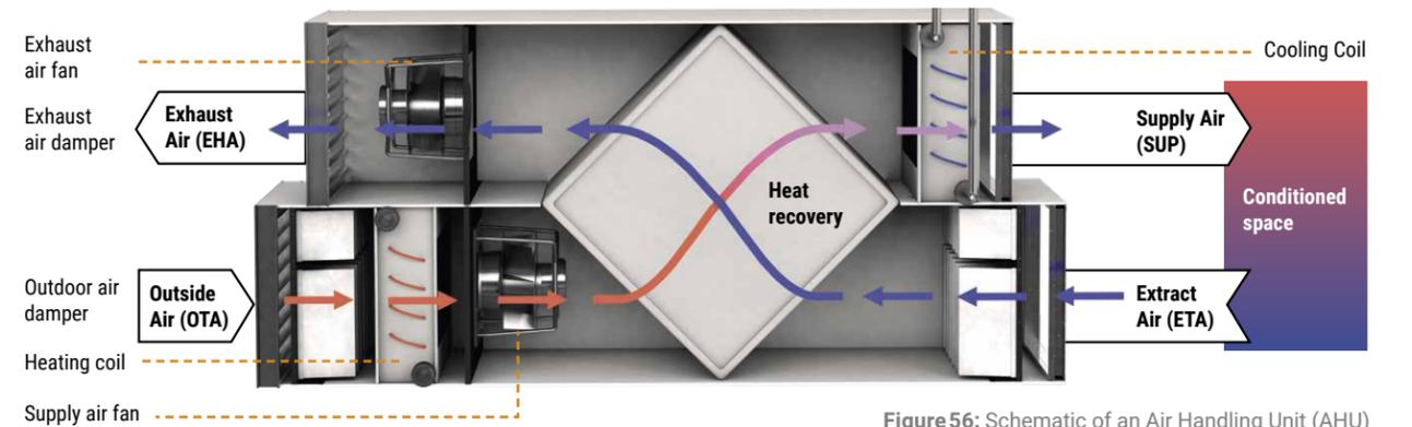
Figure 56: Schematic of an Air Handling Unit (AHU)
