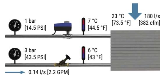
Figure 85: FCU with valve overflowing
