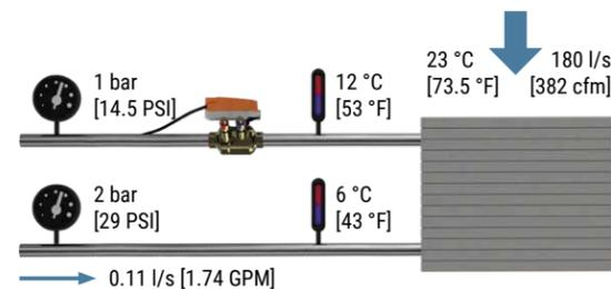
Figure 86: FCU at design operation
