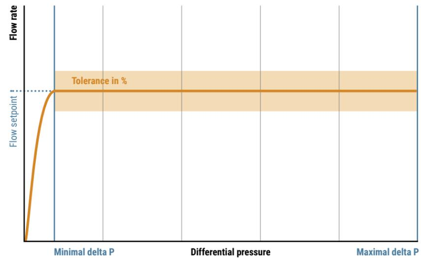
Figure 83: Dynamic Balancing of a FCU
