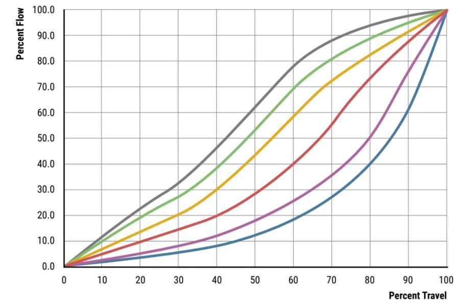
Figure 25: The distortion of the characteristic that could occur if the valve is left in position control.
