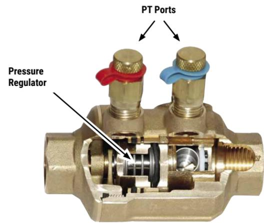
Figure 9: Components of a mechanical PI valve, example PIQCV
