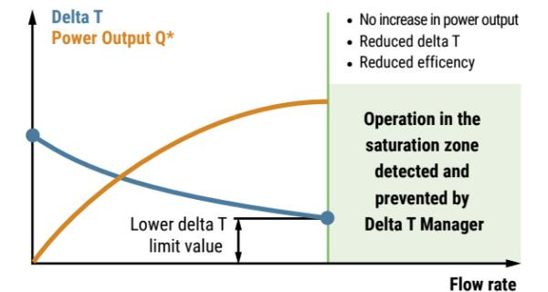
Figure 60: Improved energy-efficiency with the Energy Valves™ Delta T Manager enabled.
