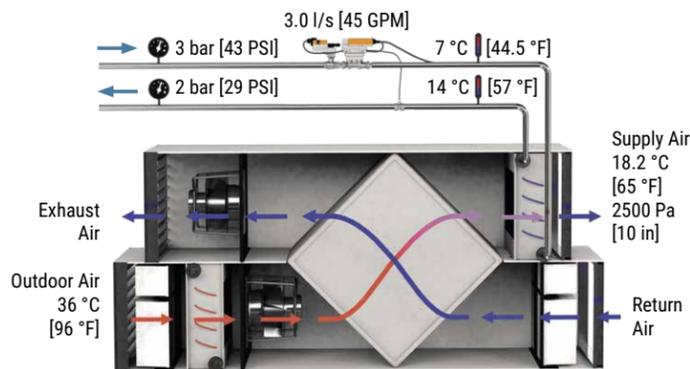
Figure 63: AHU at design operation
