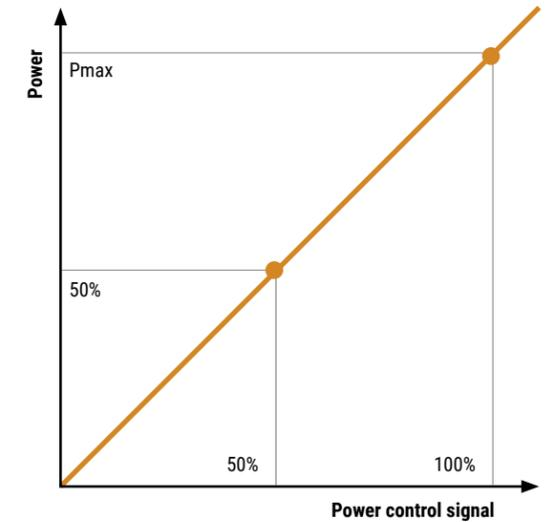
Figure 29: Control characteristics in Power Control Mode
