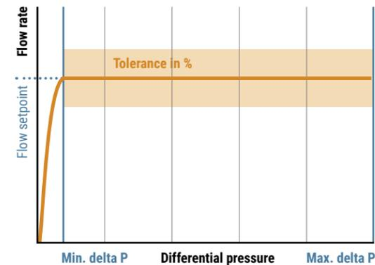
Figure 27: Control characteristics in Flow Control Mode
