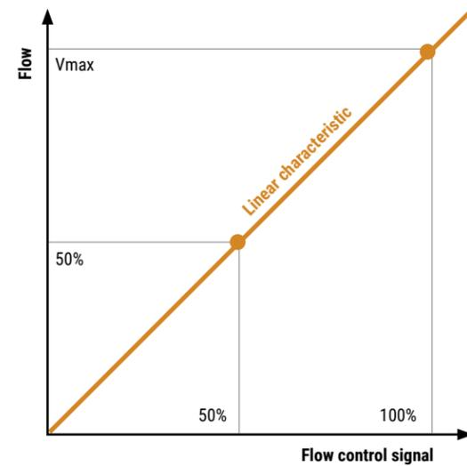
Figure 26: Flow Characteristics related to Flow Control Signal
