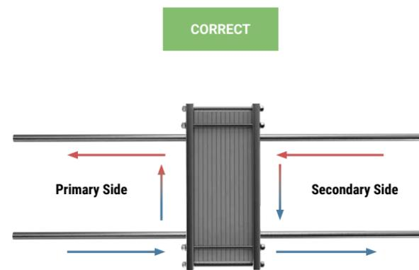
Figure 72: Cooling transfer station contraflow
