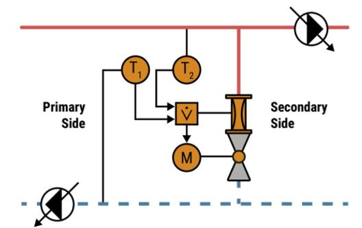
Figure 54: Shows an energy valve monitoring the temperature spread of the primary and flow through the separator.
