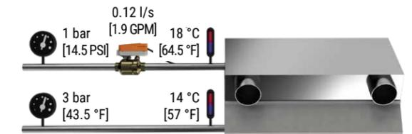
Figure 99: Chilled beam using a mechanical PI valve
