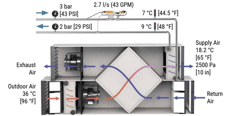
Figure 64: AHU without valve overflow
