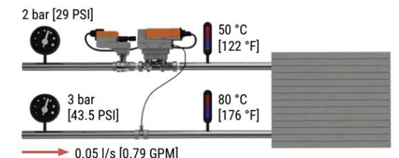
Figure 109: FCU with BMS corrected heating setpoint and required flow
