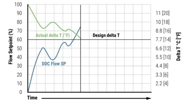
Figure 31: As the demand in the above chart starts to rise and the flow changes, the actual delta T starts to decrease
