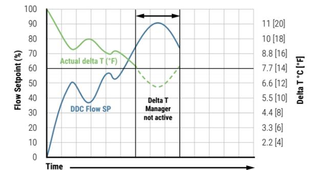
Figure 32: The above chart shows what would happen if the Delta T Manager was not active. Here the DDC setpoint drives the demand so high that the delta T will drop below the desired setpoint of 14 °F
