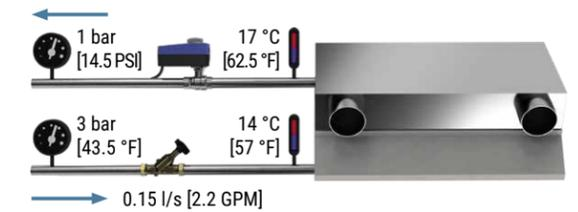
Figure 98: Chilled beam with pressure-dependent valve
