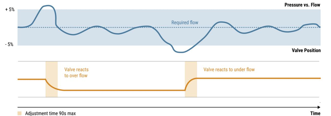
Figure 20: Reaction of ePIV to pressure changes
