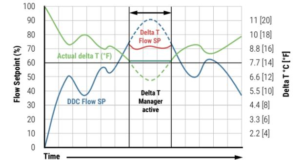
Figure 35: "Scaling Delta T Manager" scales the delta T set point depending on the current flow rate.
