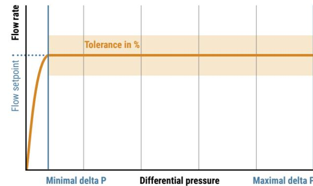
Figure 11: Improved stability with mechanical PI valves
