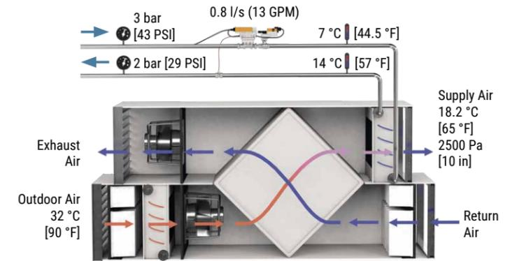
Figure 65: AHU with delta T optimized valve flow
