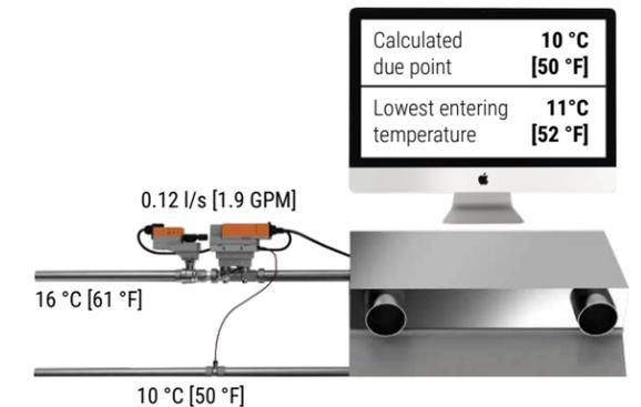
Figure 101: Chilled beam using an Energy Valve, with the BMS calculating the dewpoint with the input from a room-sensor
