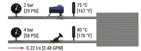
Figure 107: FCU heating conditions and pressure increase
