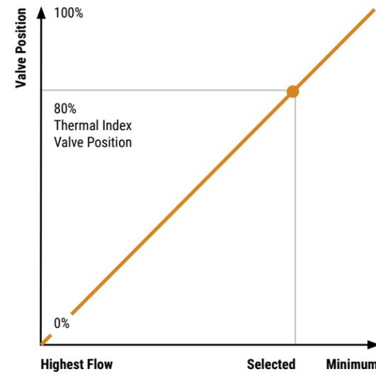
Figure 51: Shows a simple method of selecting flow temperature based on thermal index valve position.
