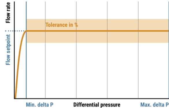
Figure 93: Dynamic Balancing of a chilled beam
