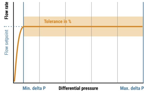
Figure 58: Dynamic Balancing assures an accurate flow rate
