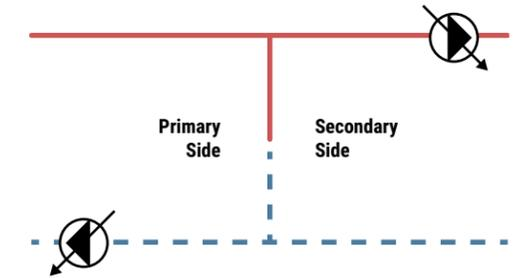
Figure 53: A simple depiction of a primary secondary circuit with an hydraulic separator.
