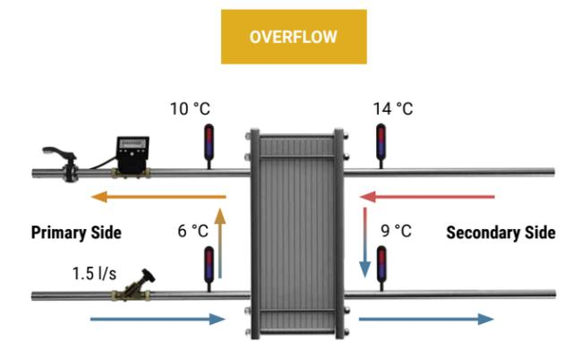
Figure 76: Overflow caused by pressure fluctuations
