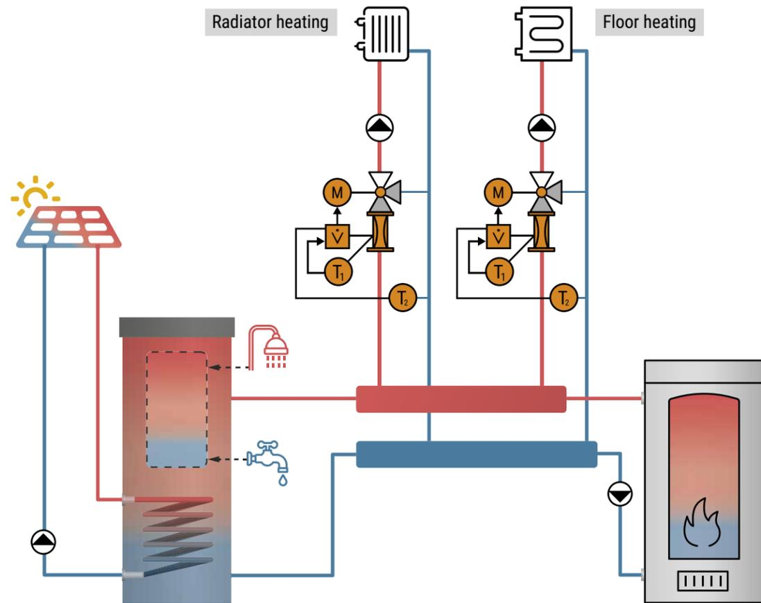
Figure 128: Typical hydronic schematic of a Central Heating Plant combining multiple alternative and renewable energy sources
