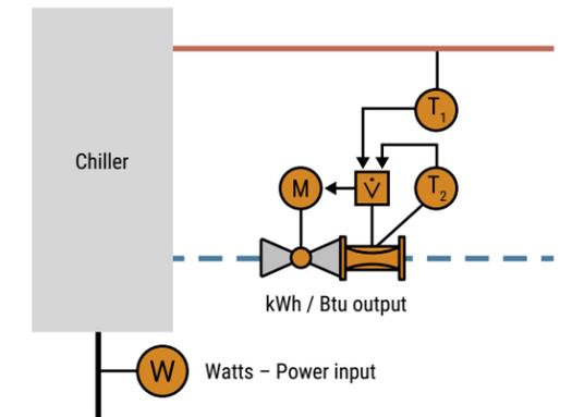
**Figure 134:** Chiller / Heat Pump with indicated cooling circuit
