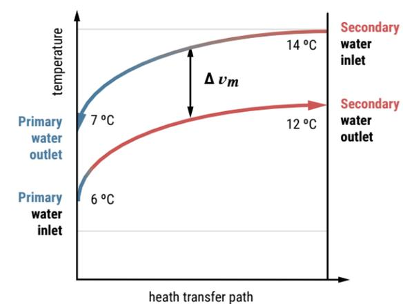
Figure 75:  $\Delta\theta_m$  average temperature difference design flow
