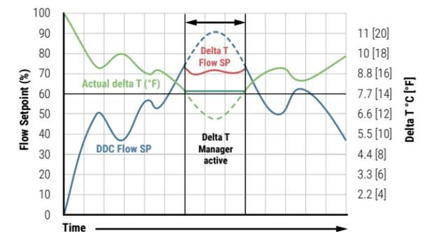
Figure 33: Delta T Manager detects low delta T, goes active, managing the flow to maintain the minimum delta T
