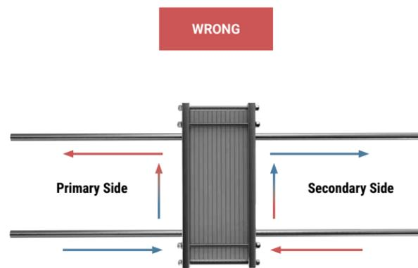
Figure 70: Cooling transfer station direct flow
