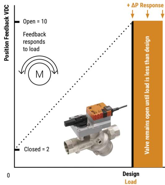
Figure 16: Pressure Dependent & Mechanical PICV
