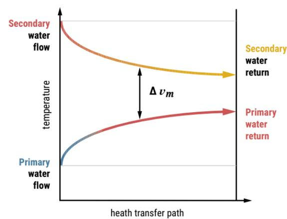
Figure 71:  $\Delta\theta_m$  average temperature difference direct flow
