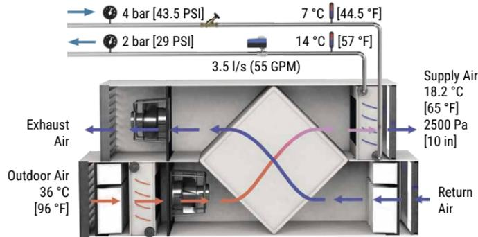
Figure 62: AHU with valve overflowing
