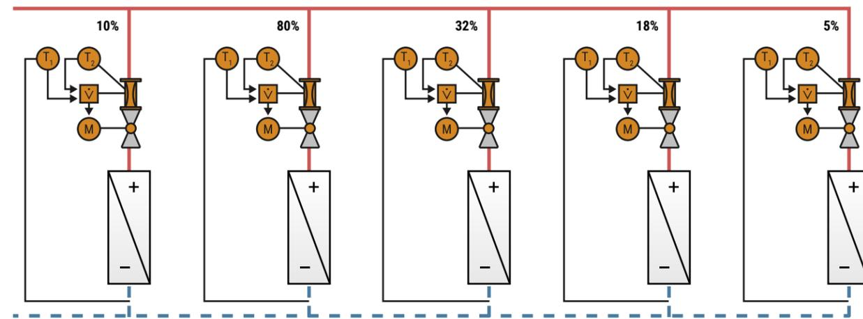
Figure 52: Shows the thermal index, the most open valve, which selected by the BMS.
