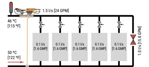
Figure 115: With an EV both leaking short-stroke valves or an open bypass can be clearly identified
