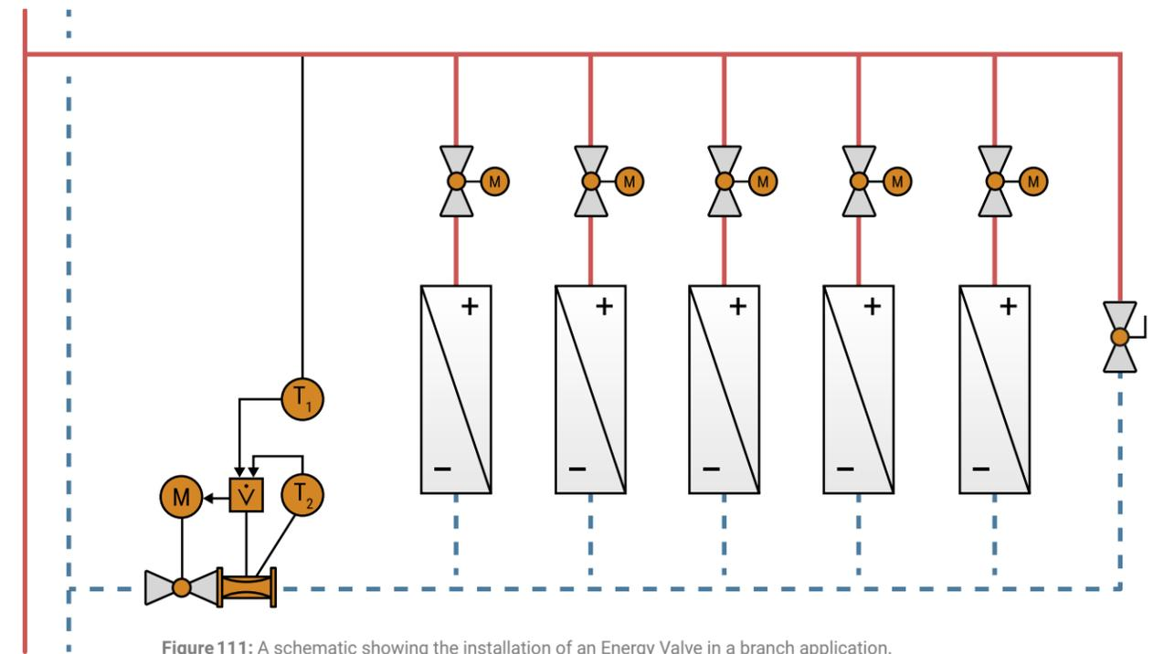
Figure 111: A schematic showing the installation of an Energy Valve in a branch application.
