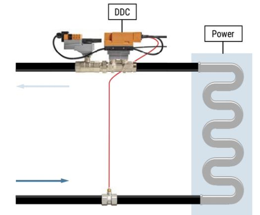
Figure 28: Power Control of the Energy input to a Consumer
